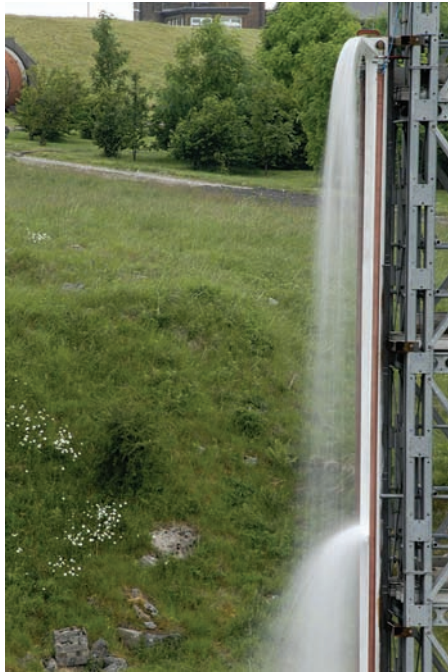
Figure 2. Intersection of free cascades from a Type A tank with a deflector plate
