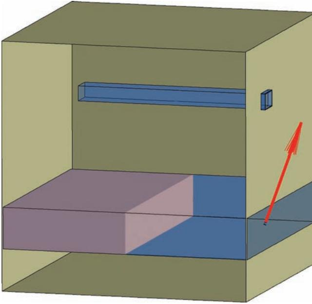
**Figure 1.** Idealised modelled geometry for an offshore platform, showing the location and orientation of a gas release from a partially-obstructed module. A HVAC duct is also shown
