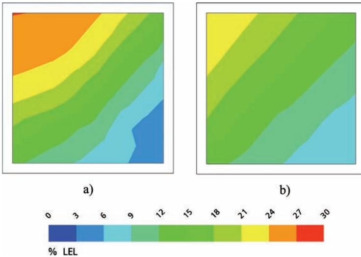
**Figure 8.** Gas concentration distribution inside the 1.5 m square 'PLQ' duct. a) 2 m inside the duct b) 6 m inside the duct
