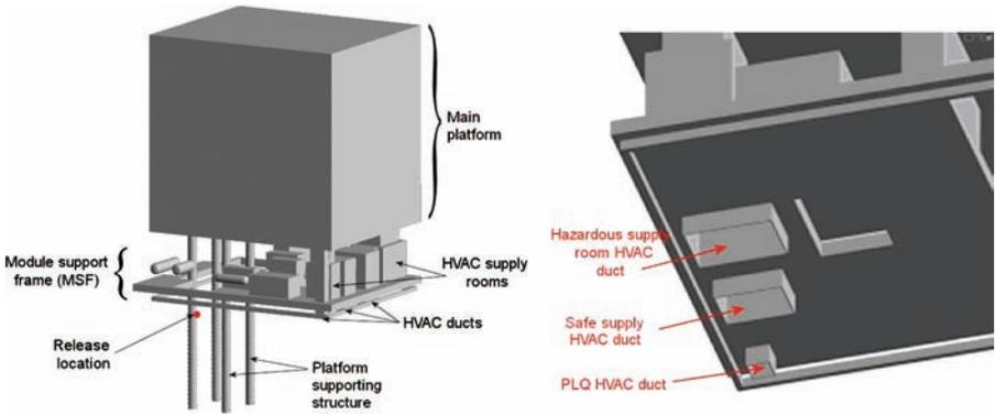
**Figure 3.** Geometry and location of HVAC inlets for the more realistic scenario
