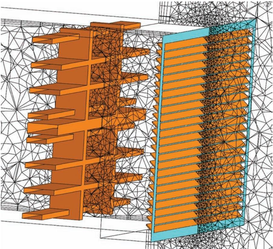
**Figure 2.** Geometry and meshing of louvres and open fire dampers at the inlet to an HVAC duct.
