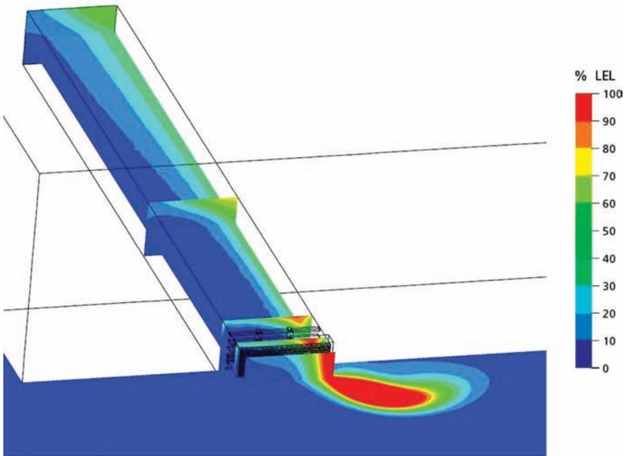
**Figure 4.** Gas concentration distribution inside and outside of an HVAC duct for a low pressure release, shown on a horizontal mid-plane of the duct
