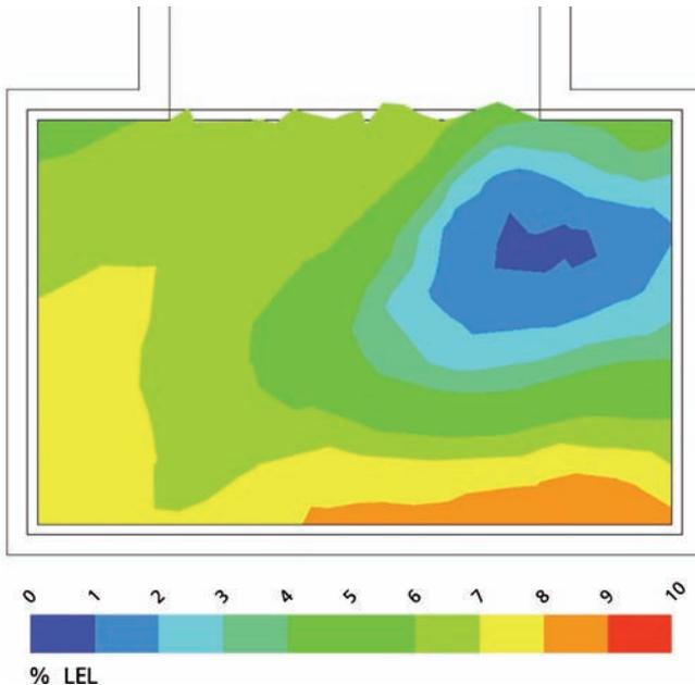
**Figure 7.** Gas concentration distribution 3.5 m inside the Hazardous HVAC inlet duct
