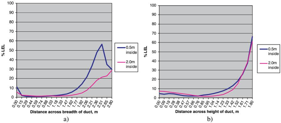
**Figure 5.** Computed gas distribution inside an HVAC duct. The location ‘0.5m inside’ is immediately downstream from the modelled louvres, the location ‘2.0m inside’ is immediately downstream from the modelled fire dampers. Also see Figure 2. a) Across the breadth of the duct b) Across the height of the duct
