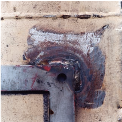
Figures 2 & 3. Close up of weld on outside and inside of case showing burnt sugar residue around weld and second area away from weld
