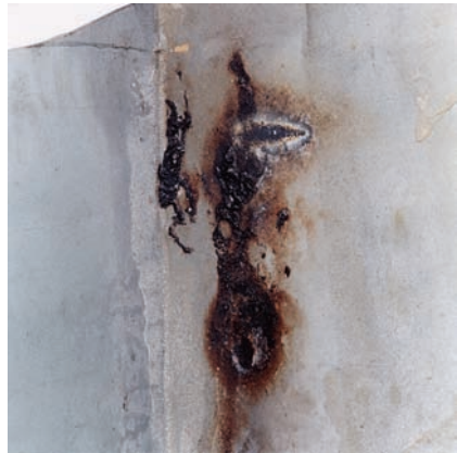
Figures 2 & 3. Close up of weld on outside and inside of case showing burnt sugar residue around weld and second area away from weld
