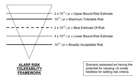
Figure 1. Sensitivity analysis example for a reactor runaway
