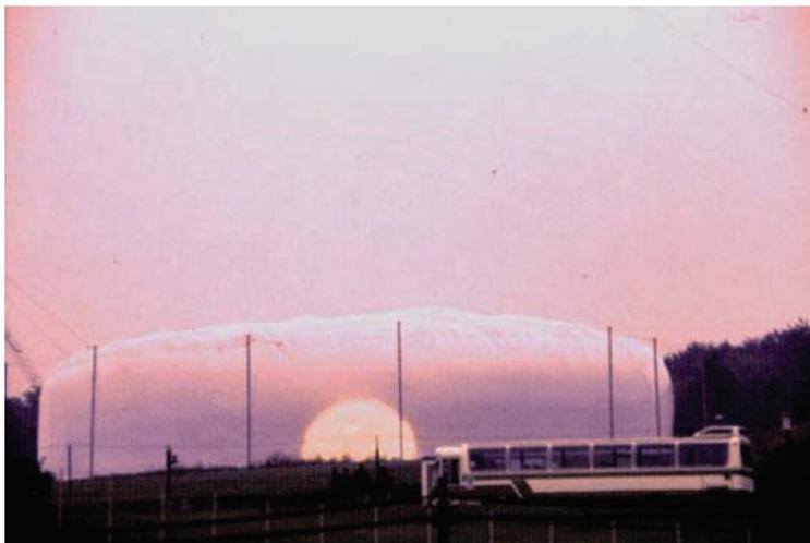
**Figure 5.** Hemispherical flame propagation in a flat, quiescent hydrocarbon air cloud
