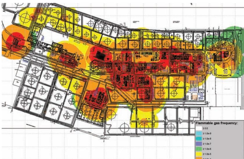
Figure 8. Base case – Frequency of flammable vapour clouds
