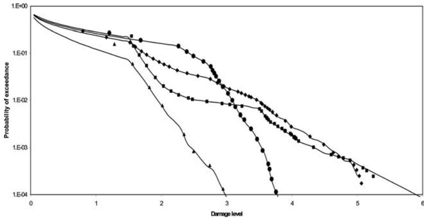
**Figure 5.** Damage exceedance curves from full explosion exceedance calculations for one unit and four nearby buildings. The points show the results of using the simplified method of calculation. These lie very close to the corresponding curves
