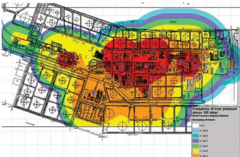
Figure 7. Base case – Frequency of overpressure above 100 mbar from site explosions
