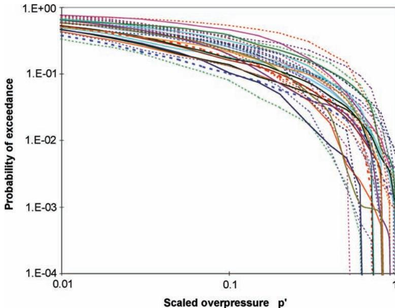
**Figure 2.** Normalised exceedance plot of UK refinery data for external releases
