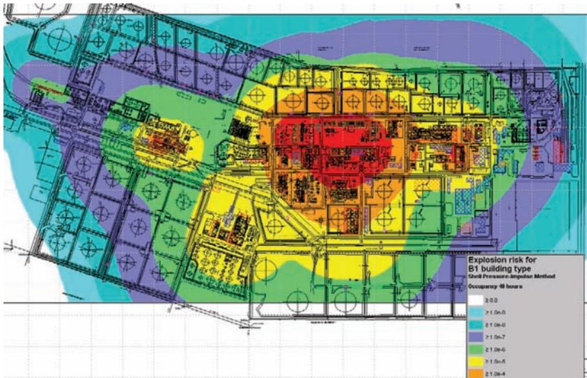
**Figure 6.** Base case – Individual risks for trailer type temporary with occupancy level of 40 hr/week
