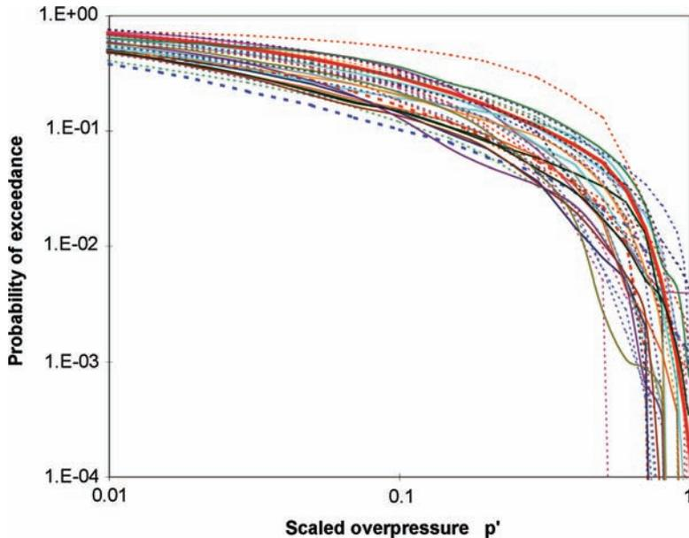
**Figure 3.** Transformed exceedance plot of UK refinery data for external releases. The heavy curve is the generic curve
