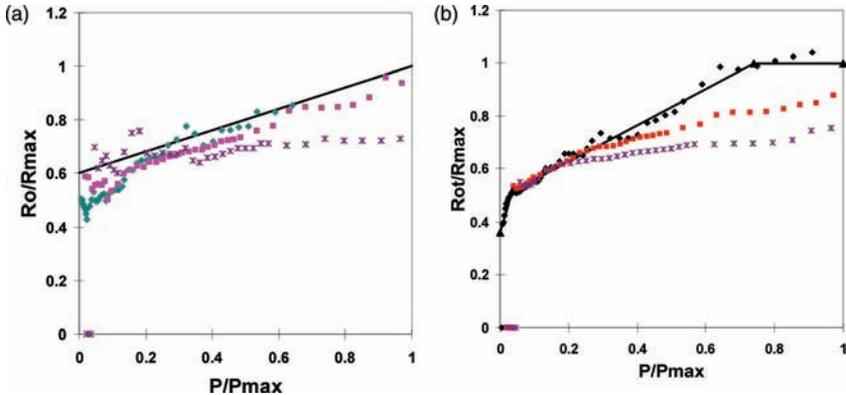
**Figure 4.** Best fit of the effective source size (effective radius  $R_o$  and  $R_{ot}$ ) for (a) overpressure exceedance and (b) impulse exceedance, derived from the UK refinery data
