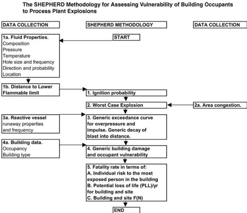
Figure 1. The simplified explosion exceedance methodology implemented in SHEPHERD
