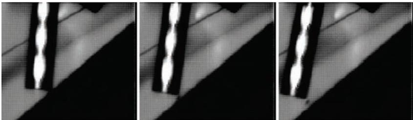
**Figure 11.** Production of a fragment during the impact of a 20 cm long steel rod on a steel target with an impact velocity of 7 m/s
