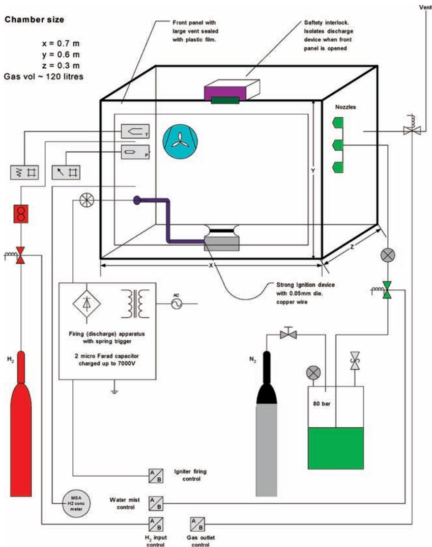
Figure 2. Schematic diagram of the strong ignition source water mist suppression apparatus
