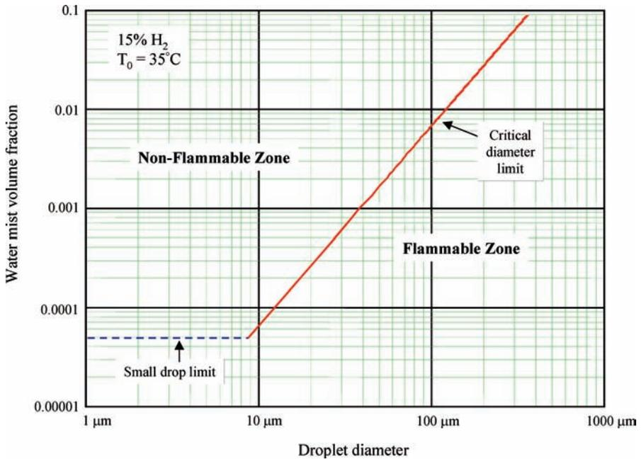
**Figure 1.** Example of a water mist inerting map constructed for a 15% hydrogen-air mixture at 35°C.
