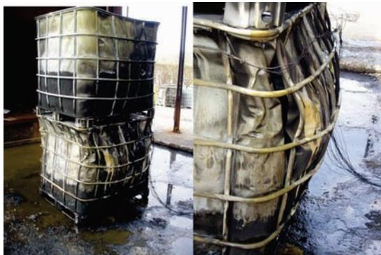
**Figure 6.** Damage to a stack of metal clad water filled IBCs during fire engulfment. Separation of metal cladding sheets is visible in lower (closeup) view
