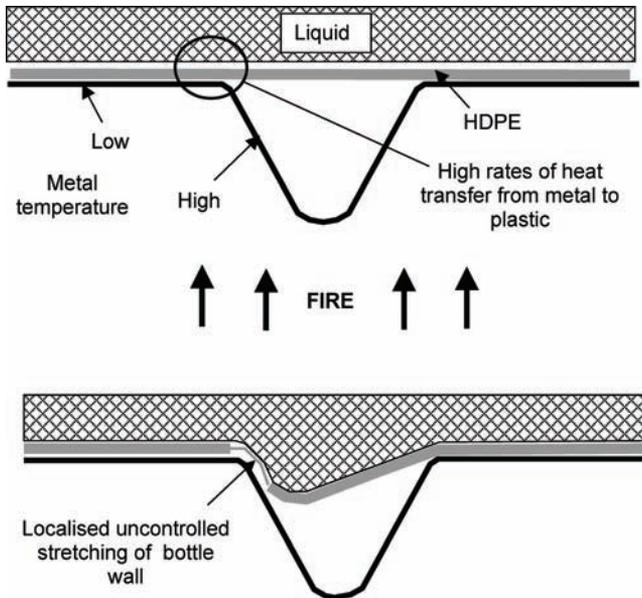
**Figure 11.** Possible mechanism of failure of HDPE inner receptacle caused by a fire under an IBC with a formed metal pallet
