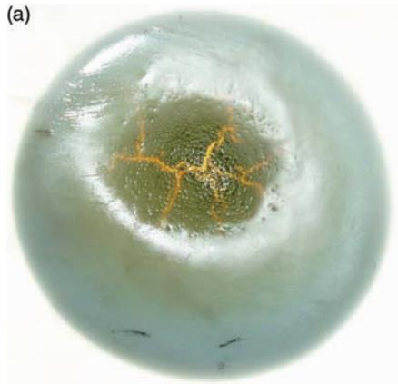
**Figure 2.** HDPE panel after water test (view from liquid side). The failure mechanism is pitting to produce holes a few hundred micron across. The characteristic leakage rate is of order 1 g/s
