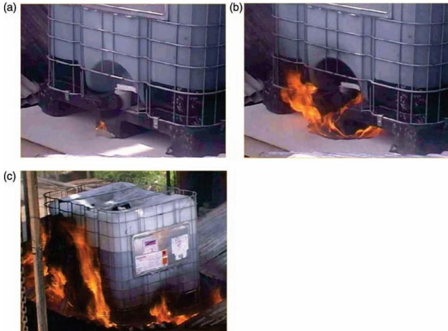
**Figure 3.** Fire in an IBC containing an industrial lubricant (flashpoint 75°C)
