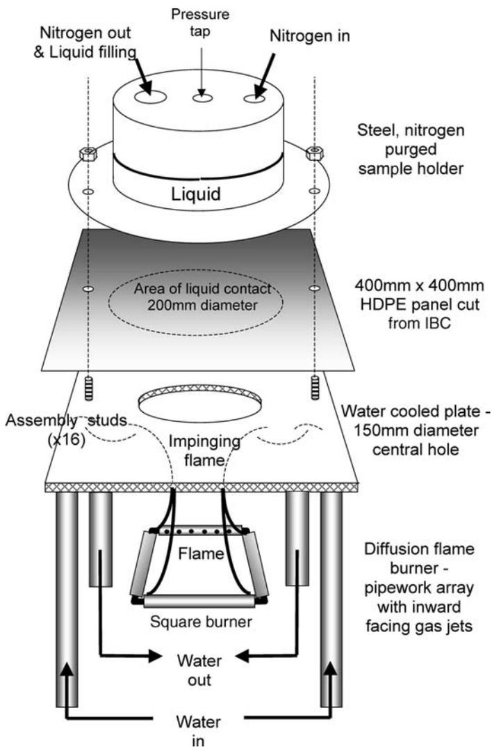
Figure 1. Reduced scale test for liquid/HDPE compatibility
