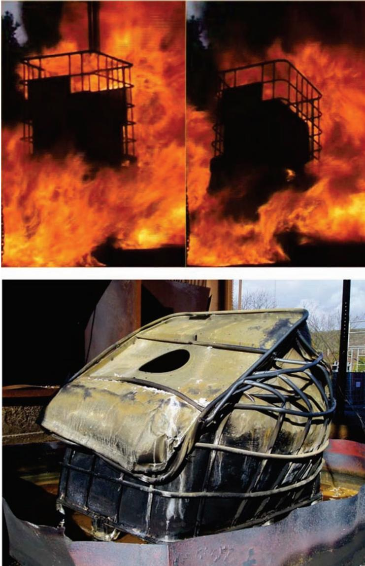
**Figure 7.** Crushing of lower (water filled) IBC by an upper IBC loaded with bricks (970 kg) during fire engulfment Above – extent of initial (arrested) yielding. Below – extent of damage following final uncontrolled collapse
