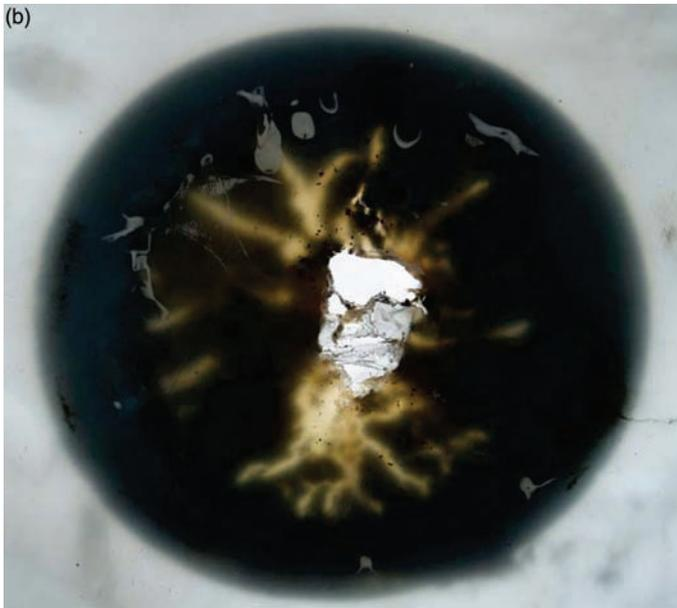
**Figure 2.** HDPE panel after diesel test (view from flame side). The failure mechanism is a large scale tear several centimetres across. The characteristic leakage rate is of order 100 g/s
