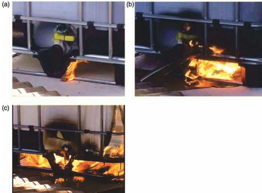
**Figure 4.** Fire in an IBC containing an industrial lubricant (flashpoint 196°C)
