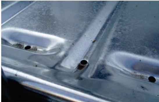
**Figure 10.** The top of a metal pallet – formed into folds to increase stiffness
