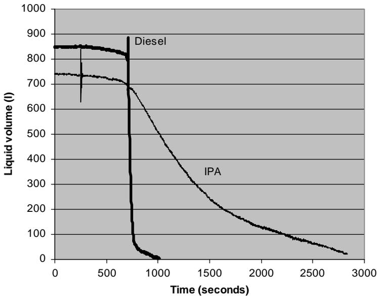
**Figure 5.** Leakage of metal clad IBCs containing Diesel and IPA. The oscillations in measured volume correspond to explosions in the ullage of the IBCs
