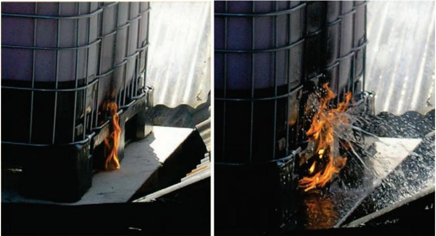
**Figure 8.** Small fire at the edge of the pallet of an IBC containing a mineral oil lubricant. Early failure occurs where flames impinge on the inner receptacle
