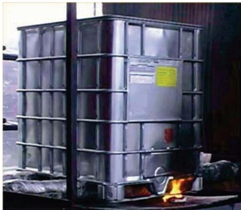
**Figure 9.** A small fire under of the pallet of a metal clad IBC containing a mineral oil lubricant. Failure of the base of the inner receptacle occurs even though this is protected by the folded metal sheet forming the top of the pallet
